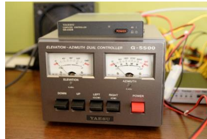
Fig. 4 YAESU G-5500 Elevation- Azimuth dual controller and YAESU GS-232B Rotator control interface
